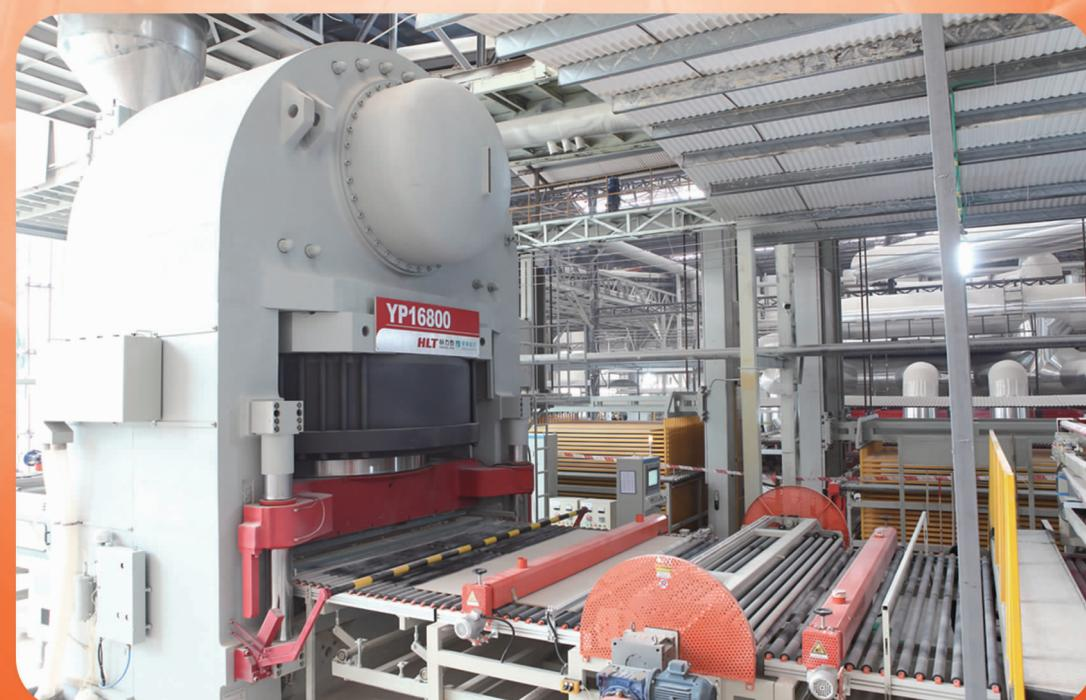
YP16800压砖机可压制: 600x1200mm, 900x1800mm,
